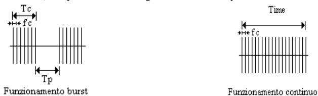
Fig. 9.2 – Rectangular current in action-pause burst operation ( T.Contr. different from “CNT”) or in continuous operation ( T.Contr. = “CNT”)
