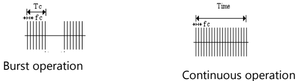
Fig. 6.3 – Rectangular current in burst operation ( T_c other than “cont”) or in continuous operation ( T_c = “cont”).
